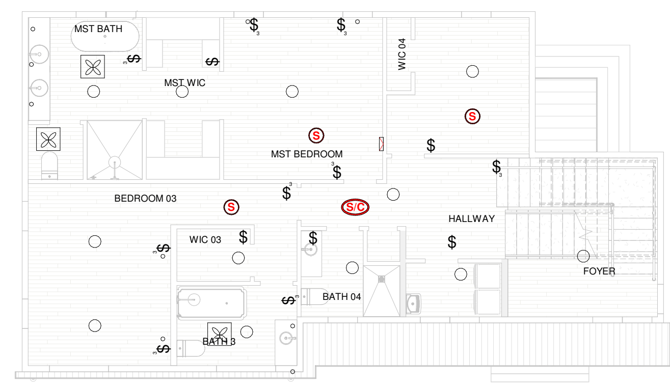
3 RCP 2ND FLOOR PLAN SCALE: 1/8" = 1'-0"
